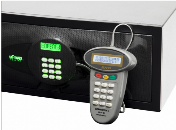
Emergency Handheld Override
